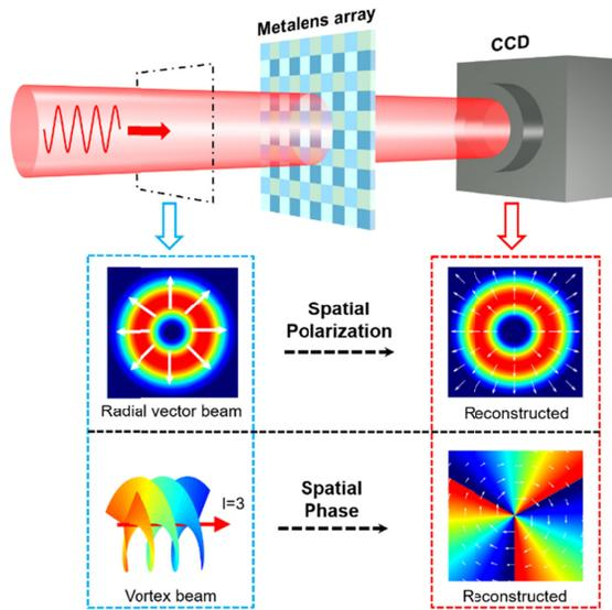
**Fig. 1.** The schematic shows the dielectric metalens-based Hartmann-Shack array for a high-efficiency optical multi-parameter detection system. The system can simultaneously measure the spatial polarization and phase profiles of optical beams. The colours are only used to enhance the clarity of the image and to distinguish metalenses with different polarization sensitivities in the array.
