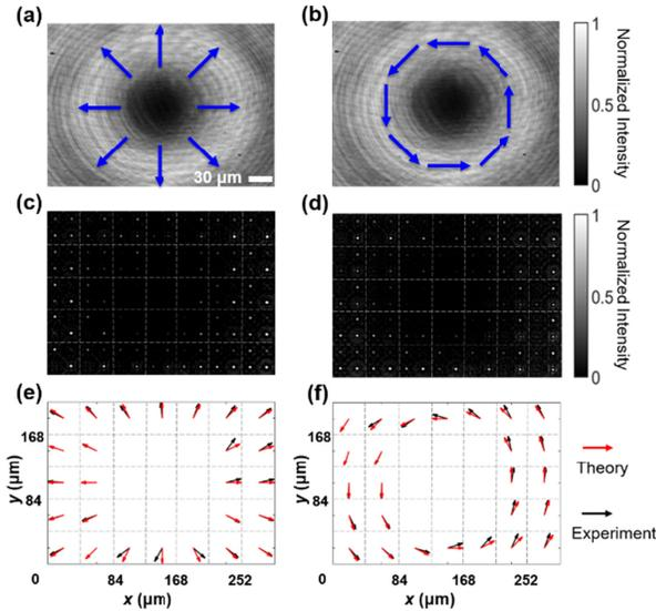
**Fig. 5.** Detection and reconstruction of two vector beams. (a, b) Intensity distributions for two vector beams. The blue arrows denote the local SOPs. (c, d) Raw data of measured focal points for two vector beams. (e, f) Reconstructed polarization profiles. The black arrows correspond to the measured local polarization vectors, and the red arrows correspond to the theoretical predictions. The dashed grey lines are drawn to identify individual pixels
