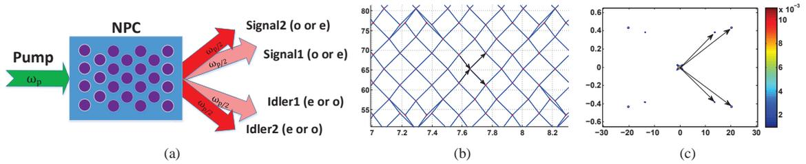
Fig. 1. (a) Schematic for the generation of path-polarization hyperentangled photon pairs. (b) Structure of the PPLN NPC. Scale is in  $\mu m$ , drawn with an aspect ratio of approximately 1:25. (c) Fourier transform  $G(\mathbf{k})$  of the PPLN NPC.
