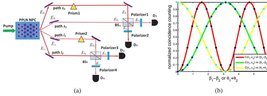
Fig. 2. (a) Experimental setup which is used to verify path and polarization entanglement.  $BS_1$  and  $BS_2$  are beam splitters with transmission coefficient  $T = 0.5$ . To verify path and polarization entanglement, we collect coincidence from detectors while adjusting prisms and polarizers. (b) Normalized coincidence counting of  $D_1, D_3$  and  $D_1, D_4$  with respect to phase modulation  $(\beta_1 - \beta_2)$  and modulation of polarizer  $(\theta_1 + \theta_2)$ .
