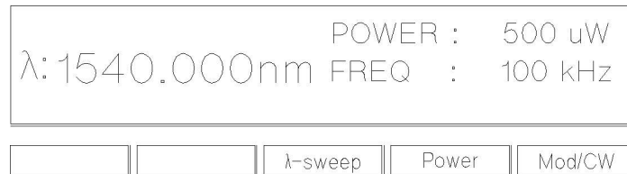
Figure 1-8. Tunable Laser Source Display after Setting Up Wavelength and Power
