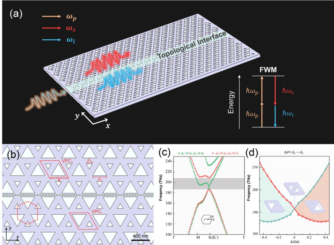
22 Fig. 1 Diagram of the on-chip VPC topological insulators. (a) Geometry of silicon-based VPCs
