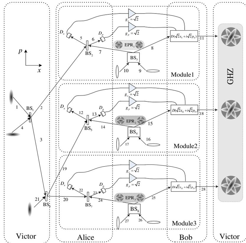
**Figure 1.** Schematic representation of quantum teleportation of CV GHZ entangled states. BS: beam splitter,  $D$ : displacement operator. The Arabic numbers denote the modes. The transmission parameter  $\eta$  of all beam splitters except  $BS_1$  is 0.5.
