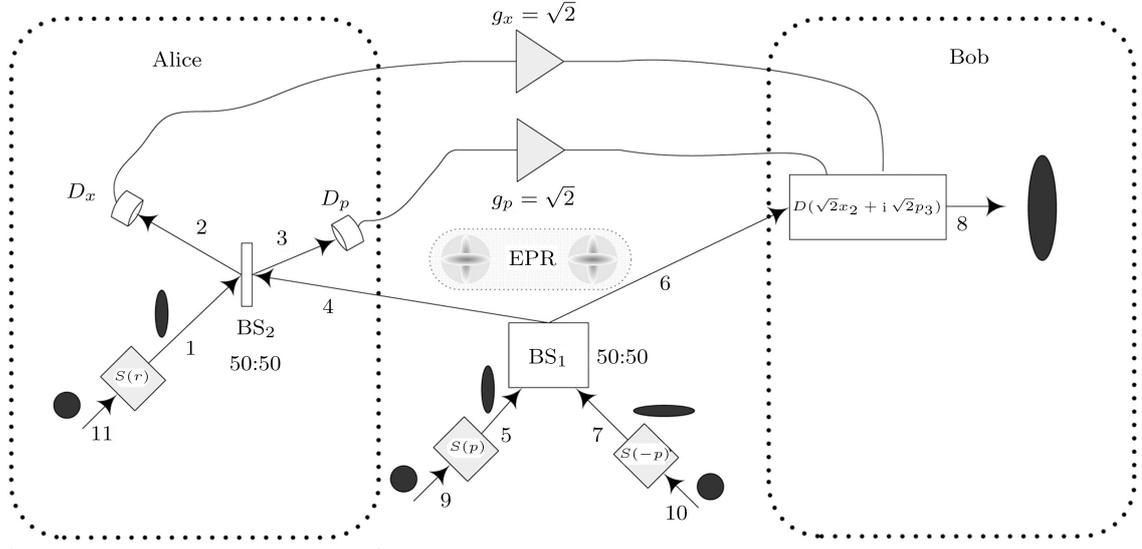
**Fig. 1.** Schematic representation of teleportation of the squeezed coherent states. The Arab numbers denote the optical modes. The  $D(\sqrt{2}x_2 + i\sqrt{2}p_3)$  denotes the displacement operator. The BS is the optical beam splitter. The  $S(r), S(p), S(-p)$  are three squeeze operators, where  $r$  is squeezing parameter and  $p$  is quantum channel parameter.
